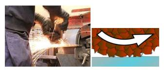
Grinding is an abrasive machining process that uses a grinding wheel as the cutting tool. A wide variety of machines are used for grinding:
